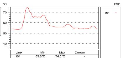
Thermal Profile Shows Intermediate Temperature Rise (74.5C ) on Connections
